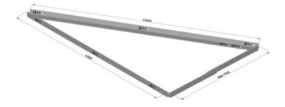
Material: Aluminum 6060 T6 Longest side: 1550 Degrees: 15°-30° Fastening: M10 double threaded screw
